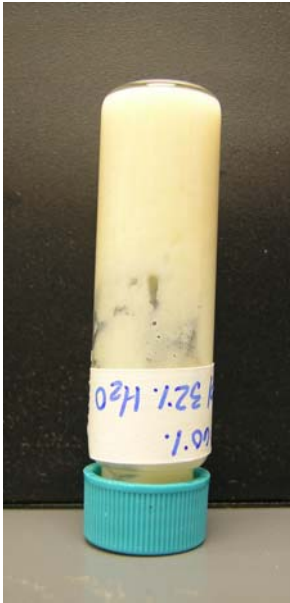
Figure 20. 8% Viscopro S.F. and 32% Tap Water in Gas Containing Ethanol
