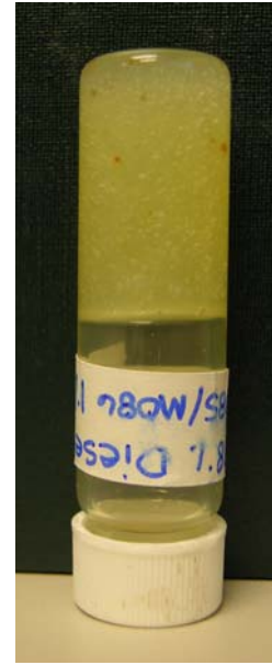
Figure 16. 1% Each MO-85M and MO-86M in Diesel Fuel
