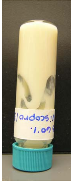
Figure 21. 8% Viscopro S.F. and 32% Tap Water in Gas Without Ethanol
