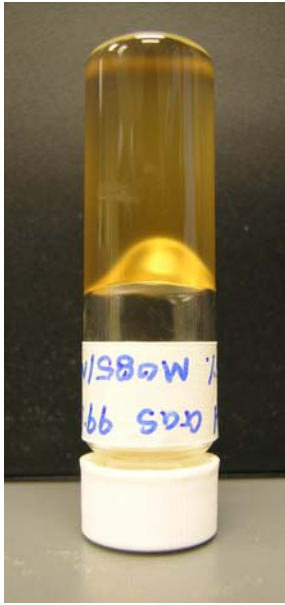
Figure 14. 1% Each MO-85M and MO-86M in Gas Containing Ethanol
