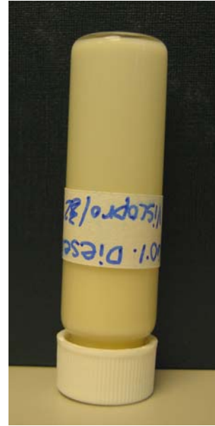
Figure 22. 8% Viscopro S.F. and 32% Tap Water in Diesel Fuel
