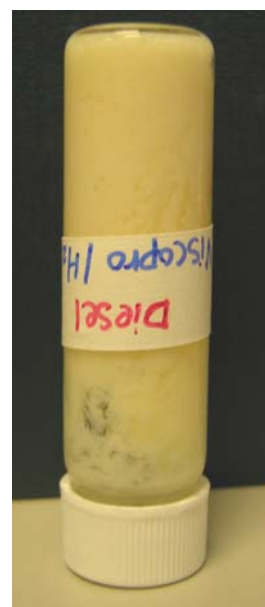
Figure 19. 16% Viscopro S.F. and 29% Tap Water in Diesel Fuel
