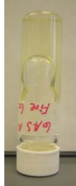
Figure 4. FireGel in Gas Without Ethanol 4-lb Simulation
