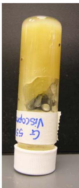
Figure 18. 16% Viscopro S.F. and 29% Tap Water in Gas Without Ethanol
